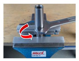
24. Pull the jet concentrator (13) from the nozzle (12), e.g. with a set of pliers.
