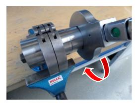
20. Lever the spiral circlip (29) out of the internal groove on the connection cover (01), by inserting the flat tip of a small screwdriver on the removal notch.
