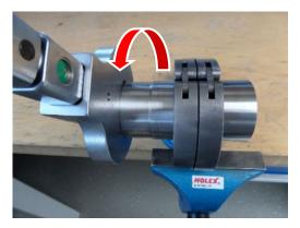
6. **NOTE** Depending on the version of the device, the threaded connection between the connection cover (01) and housing (02) is secured by a securing mechanism with two locking pins (02.1). If a locking pin (02.1) is bent several times, the material will fatigue and lose its strength.
