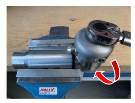
20. NOTE The set screw (34) may fall into the device when being screwed in!
