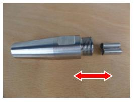
25. Remove the seal ring (13.3) from the threaded bore of the nozzle carrier (27) or from the nozzle extension (12.1) (e.g. with 0-ring pick).
