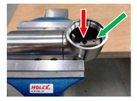
9. Secure the set screw (34) against being lost by applying a slight punch mark in the area of the front thread on the dome of the shaft-axle-connection (24).
